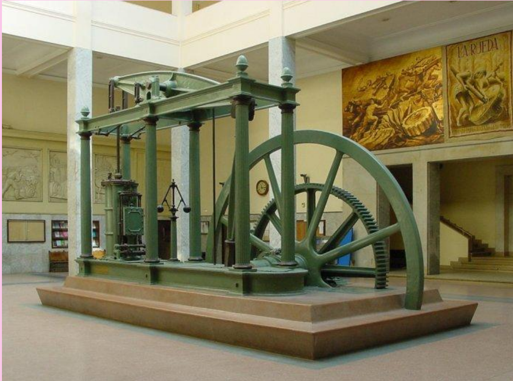
Figure 2: The Watt steam engine (1769). Notice the centrifugal regulator (sliding balls on a vertical axis) which ensures the smooth functioning of the engine, independent of variations of power solicited at the outlet. (Image: Wikipedia, the lobby of the Superior Technical School of Industrial Engineers of the UPM (Madrid))
