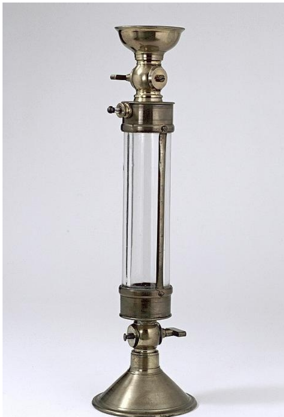
Figure 3 : Water eudiometer used by Gay-Lussac (photo by Bibliothèque de l'École polytechnique). An eudiometer is an instrument allowing the determination of the proportion of oxygen contained in atmospheric air by making it react with excess hydrogen to form water. The apparatus is placed in a water basin. Atmospheric air (or any analysed gas) is mixed with excess hydrogen and, after combustion triggered by a spark, the volume of oxygen contained in the air is determined by a one third decrease in the volume of the gas mixture accompanying the reaction.
