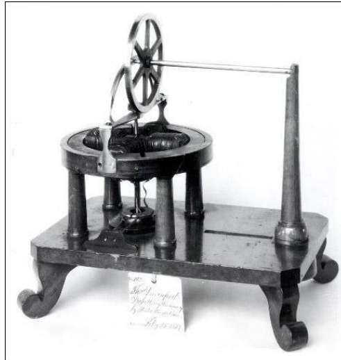
Figure 9: Davenport's motor , made of two cross coils that rotate on a vertical shaft within a wooden ring equipped with two permanent semi-circular magnets. The coils are powered by a commutator, visible at the lower extremity of the shaft (© Smithsonian Museum).
