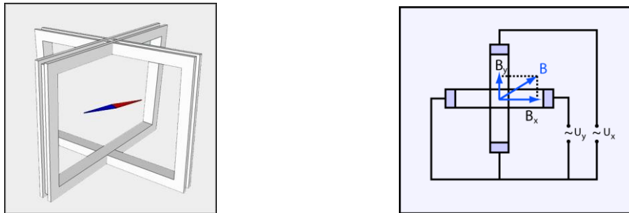
Figure A14: Rotating field and alternating current. Two perpendicular frame coils, traversed by two alternating currents phase-shifted by \pi/2 , produce a rotating magnetic field (© Ilarion Pavel).
