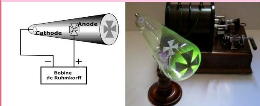
Figure 1: A Crookes tube (supplied by a Ruhmkorff coil, seen on the right). Thanks to the vacuum inside the tube, the electrons come into contact with few molecules during their trajectory and maintain the high speed acquired from the electric field (around 0.1c ). Some move beyond than the anode and this causes the glass to become fluorescent. The effect is heightened when the end of the tube is covered with a fluorescent material. The projection of the shadow of the Maltese cross led Hittorf (1824–1914) to speculate that something was moving rectilinearly inside the tube. This something would become known as a "cathode ray".
