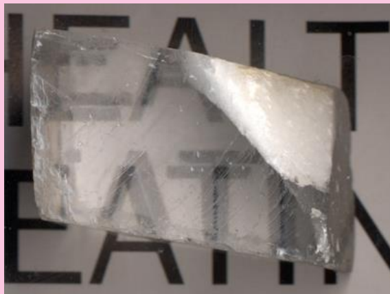
Figure 1: Double refraction through an Iceland spar crystal (calcite \text{CaCO}_3 ). The image of letters passed through the crystal is shifted in relation to the original image (effect of refraction); the image is also divided into two images (effect of double refraction).
