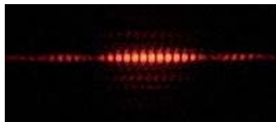
Figure 6: "Young's double-slit experiment". The wave originating from the source above, not shown in the figure (Wikipedia image, Tatoute), arrives at the double slit and produces an interference figure, the light intensity of which is shown below (Wikipedia image, Jordgette).
